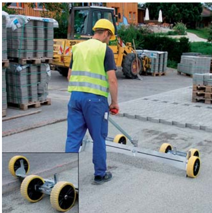
LF-125/215. bottom left: Wheel height adjustment
