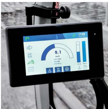
Colour LCD LED touch screen with display of real-time data and for selecting automatic programmes, driving profiles, ...
